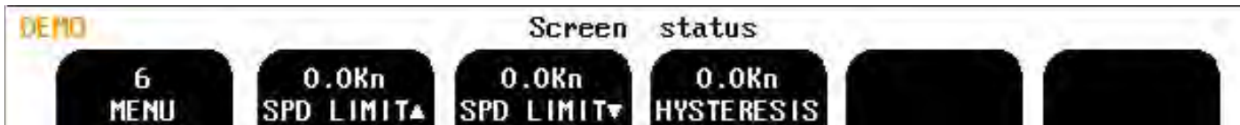
Screen status, Menu 6, speed limits and hysteresis
