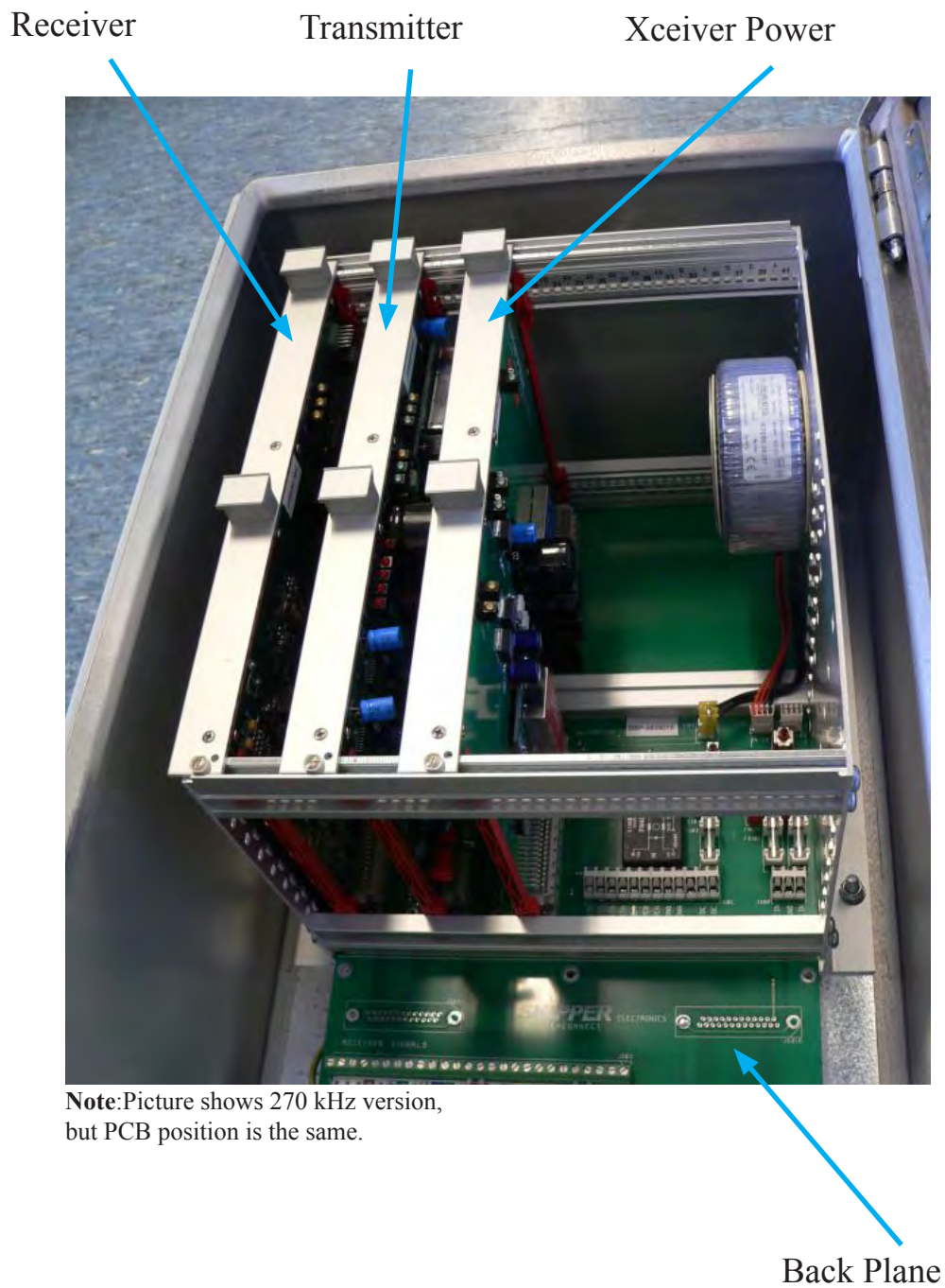
Fig. 10.1 PCB positions in Transceiver Unit
